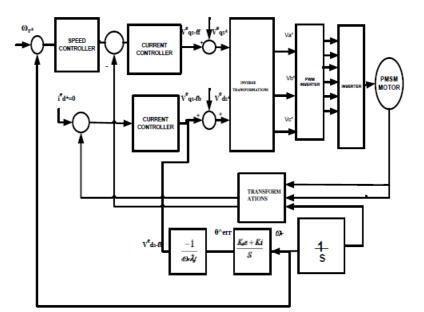
Fig.1 Overall block diagram of existing sensorless control system
