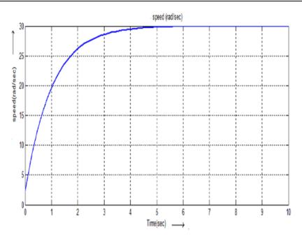
Fig.14 Actual rotor speed of PMSM for low speed operation(300rpm set speed)
