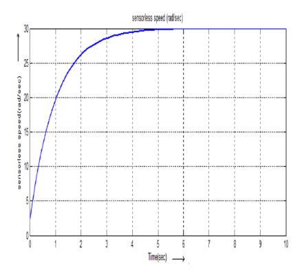
Fig.15 Estimated rotor speed of PMSM for low speed operation (300 rpm set speed).
