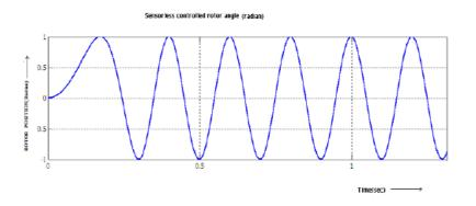
Fig.11 Estimated rotor angular position for 300 rpm set speed using hysteresis current controller.
