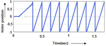
Fig.8 Actual rotor angular position for 300 rpm set speed using PWM VSI control
