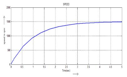
Fig.18 Actual rotor speed of PMSM for high speed operations (1500 rpm set speed) using hysteresis current control.
