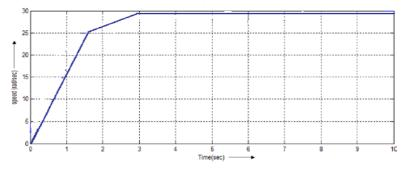
Fig.12 Actual rotor angular position for 300 rpm set speed using PWM VSI control
