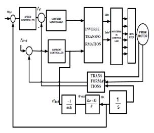
Fig.4 Proposed sensorless system block diagram
