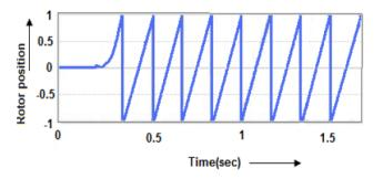
Fig.9 Estimated angular position for 300 rpm set speed using PWM VSI control
