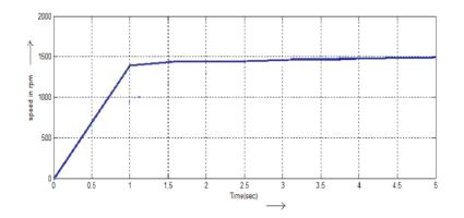
Fig.16 Actual rotor speed of PMSM for high speed operation (1500 rpm set speed) using PWM VSI control.
