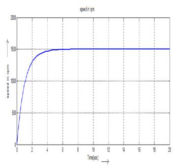
Fig.19 Estimated rotor speed of PMSM for high speed operations (1500 rpm set speed) using hysteresis current control.
