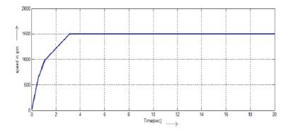
Fig.17 Estimated rotor speed of PMSM for high speed operation (1500 rpm set speed) using PWM VSI control.
